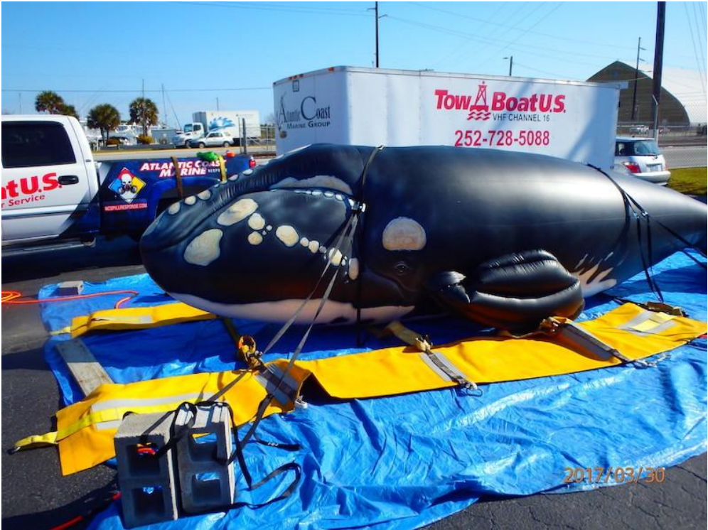
Figure B4. Straps have been positioned under the whale by simulated boat salvage techniques, and lift bags positioned and attached on either side of the whale. Note: encircling straps and cinder blocks prevent the inflatable whale from blowing away and are not a part of the proposed rescue method.
