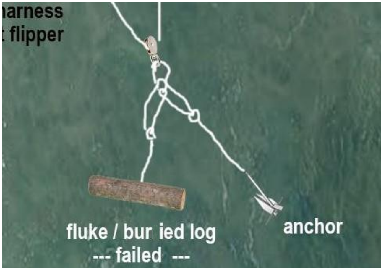
Figure A2. Close-up of the anchored pulley system that helped to redirect the whale back towards the water (diagram courtesy of SR 3 )
