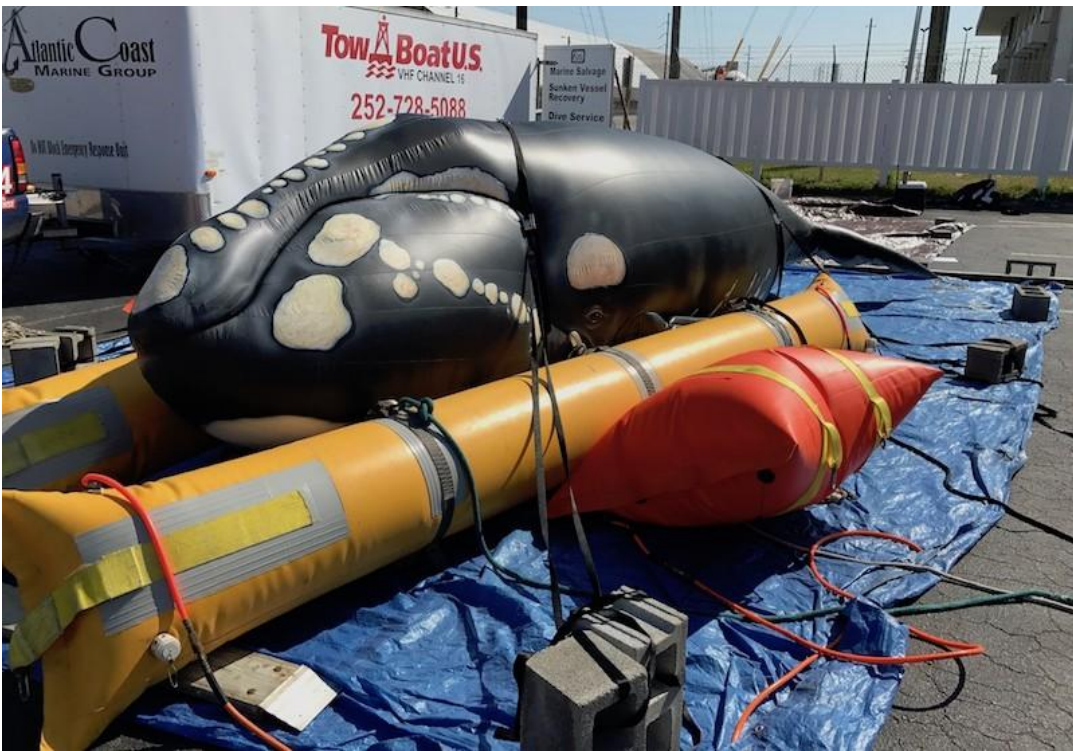
Figure B6. Front angle view of the previous image. Note: encircling straps and cinder blocks prevent the inflatable whale from blowing away and are not a part of the proposed rescue method.
