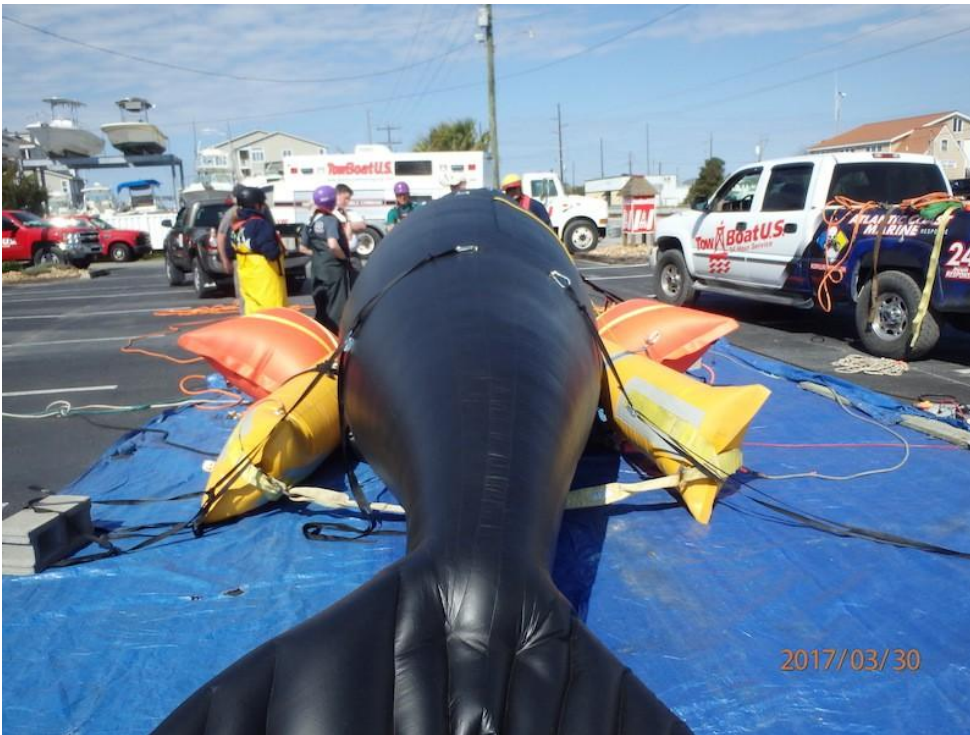
Figure B5. Lift bags are inflated on either side of the whale, forming a sling with the straps beneath the whale. At this stage, the floats could be pulled sideways initially to free the whale from underlying substrate and shallows, then pulled forward, then rapidly purged to fall away and allow the whale to swim free. Note: encircling straps and cinder blocks prevent the inflatable whale from blowing away and are not a part of the proposed rescue method.
